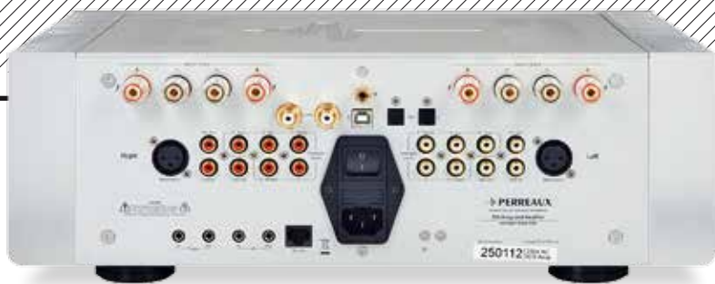
ABOVE: No fewer than five line inputs (one balanced on XLR) are joined by MM/MC, a preamp out/main amp in and a fixed tape output (all on RCAs), plus 4mm speaker terminals. There are also four S/PDIF digital ins (two coax/optical) and a USB Type-B
